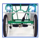
The "Wide Track" front wheel base design provides greater lateral stability in turns.
