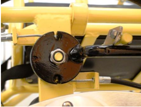
Properly mounted brake arm
